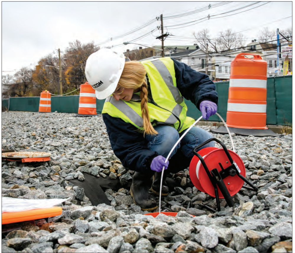
Stefanie Paige collects measurements at a groundwater well on the main Garfield Avenue site.
